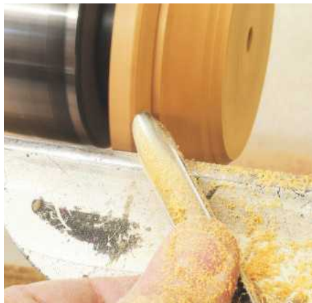
▲ Pic.11 The edge bead is rolled over using the wing of the gouge. The beads on a cross-grain piece like this are turned the opposite way to spindle work
